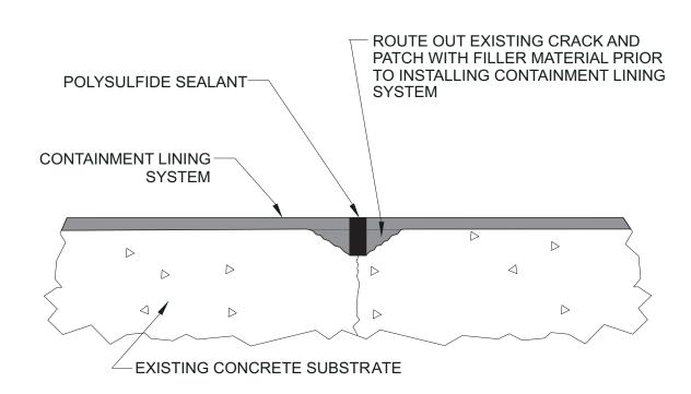
NOTE: USE SERIES 201, 237SC, 239SC 100% SOLIDS EPOXY MIXED WITH FINE AGGREGATE CREATING A MORTAR MATERIAL TO FILL ROUTED OUT AREA. FLEXIBLE JOINT SEALANT WIDTH TO DEPTH RATIO SHOWN IS APPROXIMATELY 2:1. DETAIL CAN BE BUILT BY INSTALLING CONTAINMENT LINING SYSTEM OVER FILLER MATERIAL, RESAWCUTTING, AND INSTALLING SEALANT.
