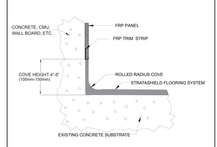
NOTE: USE DRY MIXED TROWELABLE MORTAR VERSION OF FLOORING MATERIAL TO BUILD COVE AND BASE.
