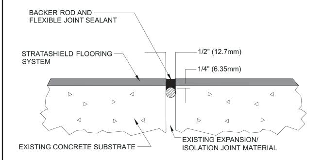
NOTE: FLEXIBLE JOINT SEALANT WIDTH TO DEPTH RATIO SHOWN IS APPROXIMATELY 2:1. DETAIL CAN BE BUILT BY INSTALLING FLOOR SYSTEM OVER JOINT, RESAWCUTTING, AND INSTALLING BACKER ROD AND SEALANT.
