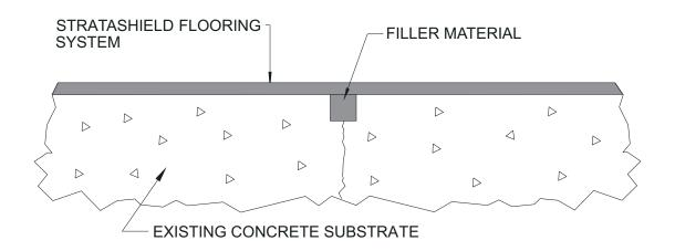
NOTE: USE SERIES 215 OR STRATASHIELD 100% SOLIDS EPOXY MIXED WITH FUMED SILICA, SILICA FLOUR OR FINE AGGREGATE FOR FILLER MATERIAL
